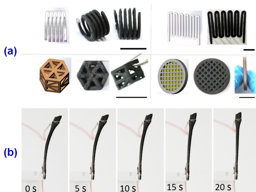
Figure 12. (a) Conductive structures of multi-walled carbon nanotube (MWCNT) nanocomposites and original resins. (b) Shape memory effect of the MWCNTs nanocomposites prepared by DLP 3D printing (ohmic heating process). Reprinted with permission from Ref. [101] Copyright 2017 Elsevier and Copyright Clearance Center.
