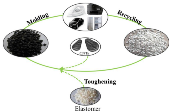
Fig. 1. Schematic diagram of recycling, functionalization and reuse of PBT materials.
