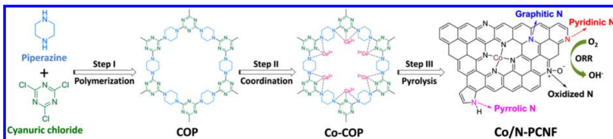
Figure 1. Schematic of the preparation of cobalt, nitrogen dual-doped porous carbon nanosheet-assembled flowers (Co/N-PCNF).
