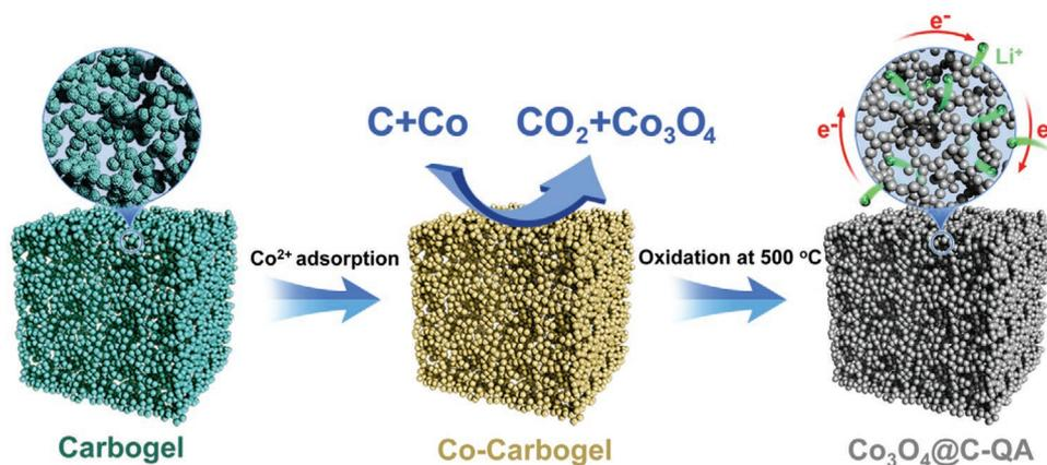
Figure 1. Schematic diagram of the preparation procedures of the Co<sub>3</sub>O<sub>4</sub>@carbon quasiaerogels (Co<sub>3</sub>O<sub>4</sub>@C-QA).
