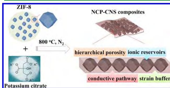
Figure 1. Schematic illustration of the formation of the NCP–CNS composites.
